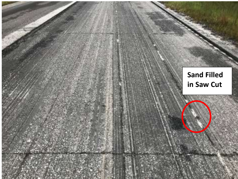
FIGURE 1 Deep saw cuts to simulate pavement cracks.
