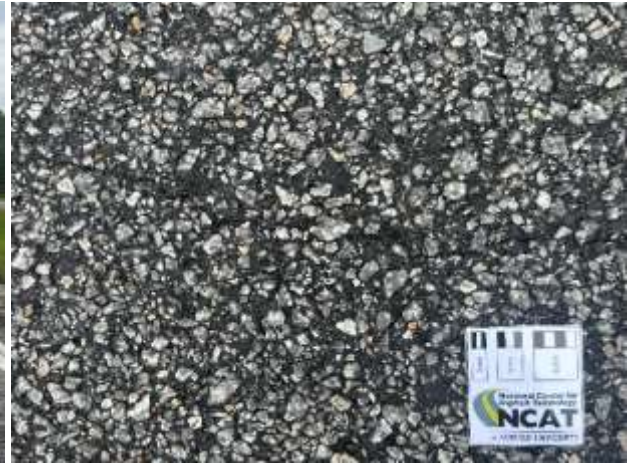
E6A (87.8% of G_{mm} ) representative cracking
