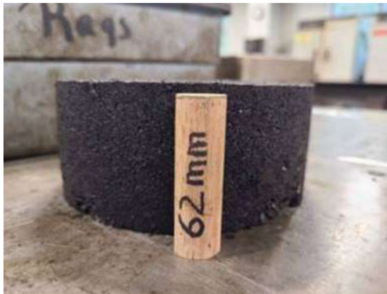
FIGURE 15 Typical expansion with RTR specimens.
