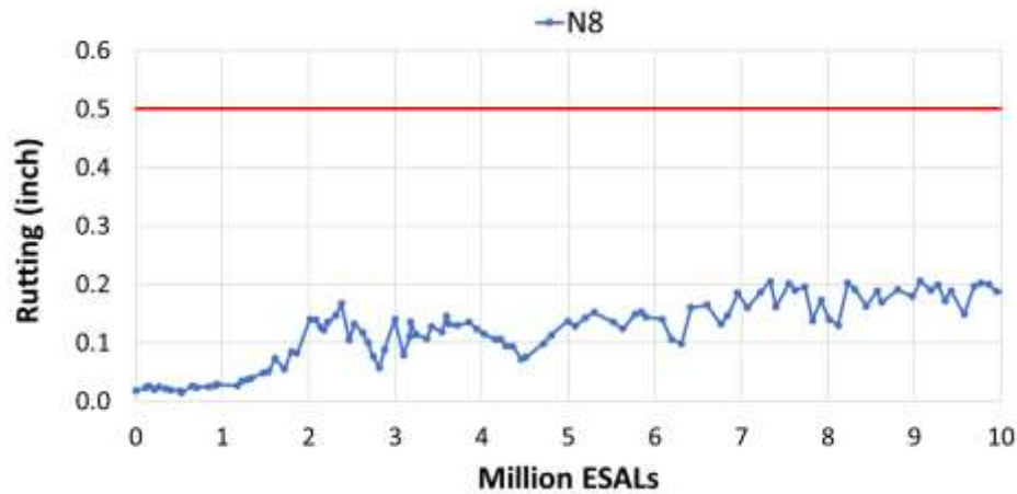
FIGURE 12 Field rutting data of Section N8.
