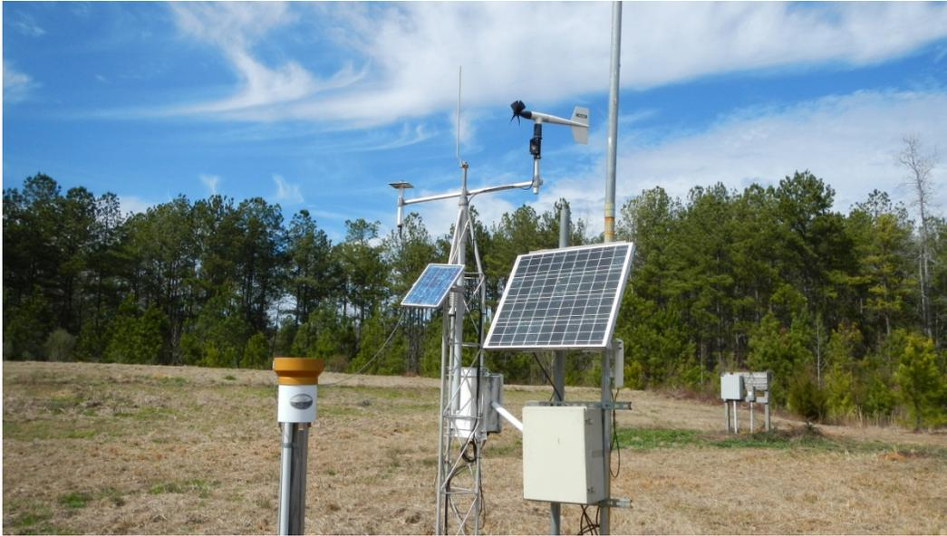
**Figure 28 Test Track On-Site Weather Station**
